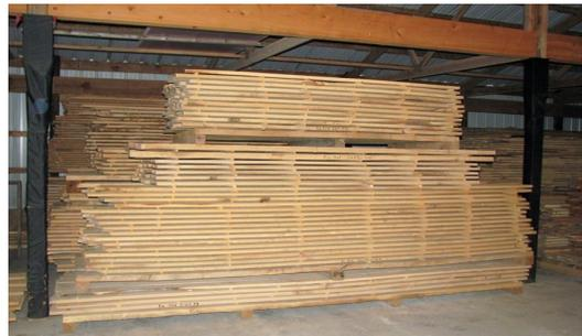
Showing proper stacking of a stickered pile
