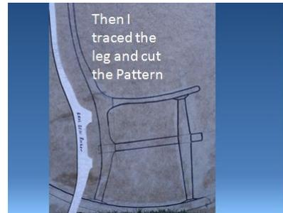
6. Here we see the first scaled drawing of Dick's newest chair drawn full scale on a 4 x 4 hard board.
