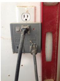
He also demonstrated a switch unit he bought at Sears that simultaneously starts the vacuum connected to his miter saw at the same time he starts the saw and delays the stopping of the vacuum a few seconds after the saw stops. I believe the unit only cost about \$12 or something like that. It also has additional outlets to support the operation of a light or other accessories as needed.
