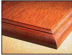
When applying liquid stains, the stain soaks more deeply into the pores of the end grain than the face grain, darkening the ends much more than the faces, see photo above.
