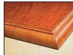
In the photo above, the face is sanded with 220-grit and the end grain with 600-grit, resulting in a much better color match.
